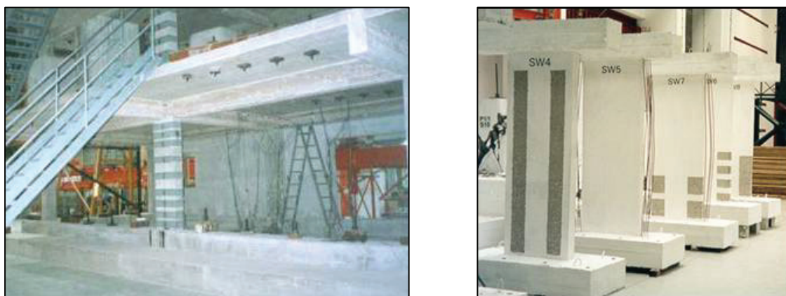
Figure D-2 Application of selective intervention on RC walls and full scale frame
