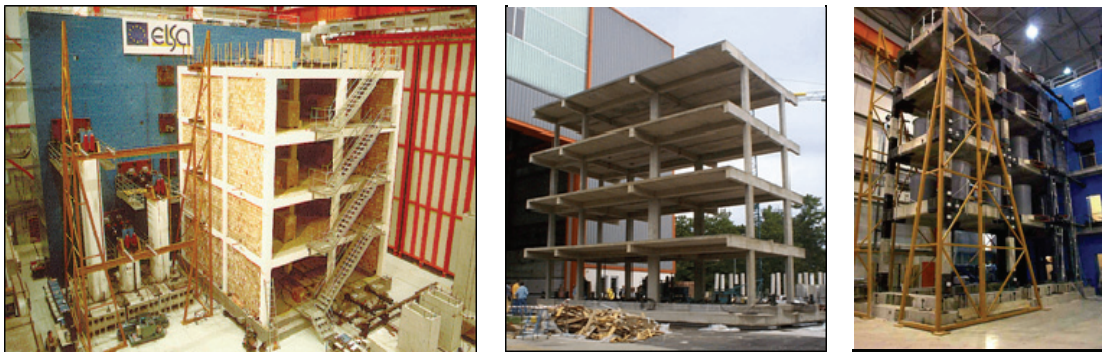
Figure D-1 Full scale testing of infilled frame, bare RC and composite frame at JRC Ispra, Italy
